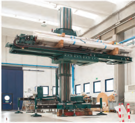
Loading and lifting test (Dummy weight)
